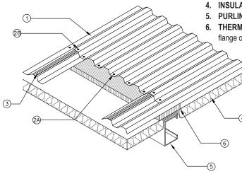
CONSTRUCTION NO. 244 (WITHOUT THERMAL BLOCKS) BERRIDGE DEEP DECK PANEL THROUGH 4" BLANKET INSULATION INTO OPEN PURLINS
