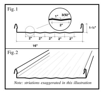
From an aesthetic point of view, the use of subtle striations is distinctly superior to the introduction of pencil ribs, grooves or other more obvious corrugation or roll forming process; In fact the striations in installed *RIGIDPRO*-FILE Cee-Lock panels are virtually undetectable. Best of all, panels with mild striations exhibit virtually no "oilcanning", buckling or waviness.
