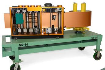
The Berridge Model SS-14 Portable **Roll-Former forms continuous**length, eave-to-ridge straight Berridge Tee-Panels, and Curved Tee-Panels. The Berridge Model SS-14 Portable Roll Former also curves
