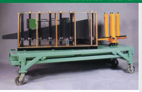
A single-leg machine, designed to form the Tapered Tee-Panel or Tapered High Seam Tee-Panel using coil widths up to 23-7/8". After one leg is formed, the pan is cut to the desired tapered shape, then the second leg is formed by running the panel back through the roll former. The resulting Tapered Tee-Panels are used for conical shaped roofs.
