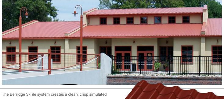
The Berridge S-Tile system creates a clean, crisp simulated tile appearance with prefinished metal. The continuous, up to 40' long, eave-to-ridge panels provide fast installation without endlaps and are only 1.2 lbs/ft² providing a professional, high-end look with minimal weight and installation expense.
