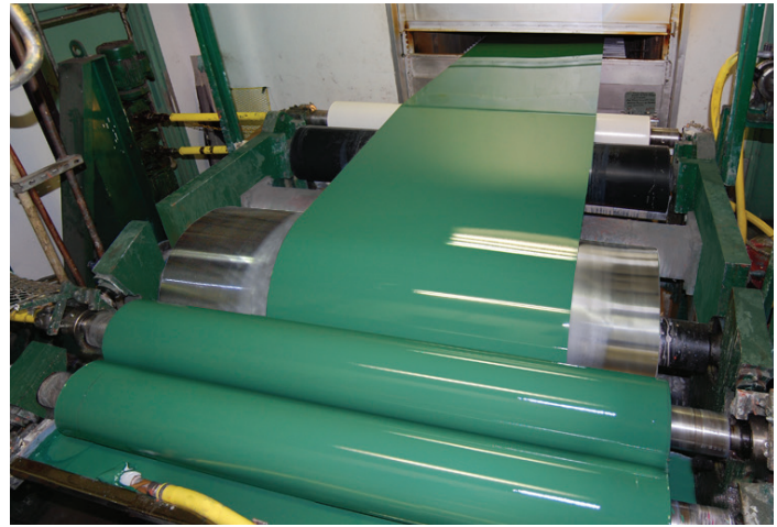
Berridge owns and operates its own modern continuous coil coating line in San Antonio, Texas, painting both 48" and 42" wide master coils.
