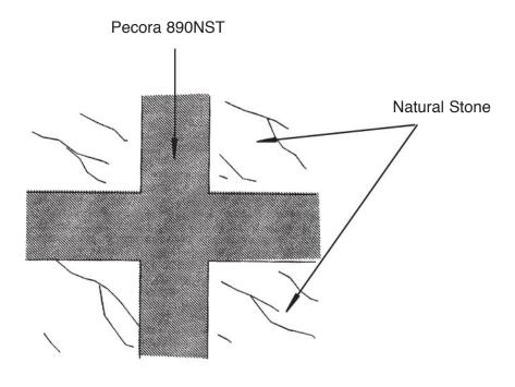
Sealant should be applied in a continuous operation using sufficient pressure to fill the joint and make complete contact to the joint sides. Tool the sealant slightly concave using solvent or dry-tooling techniques. Contact Technical Services prior to tooling with solvent. Do not tool with soap or detergent and water solutions.
