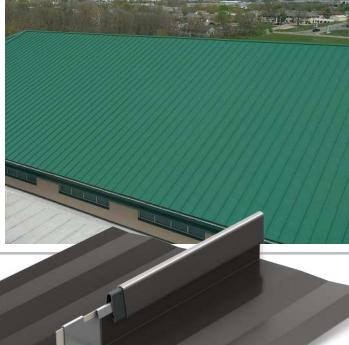
Providing a taller seam option, an additional finish option and wider coverage than the Tee-Panel, the Berridge High Seam Tee-Panel is designed to provide additional options for creating stunning residential or commercial designs over solid sheathing. This 1" or 1½" high panel can be used for straight or curved applications.\*
