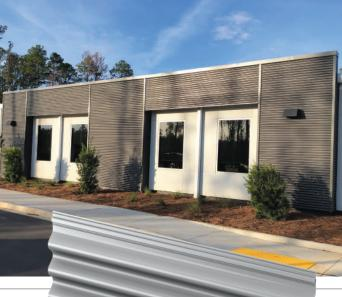
The Berridge HC-16 Panel is a concealed fastener 7/8" deep corrugated metal wall panel which can be installed horizontally or vertically and can interlock with Berridge's BR-12, HR-4, HR-16, HS-8, HS-12, and the Reveal Series panel profiles for maximum design flexibility.
