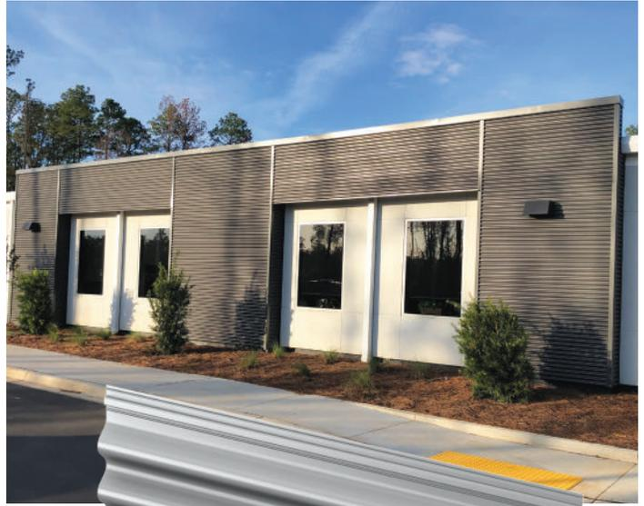
*The Berridge HC-16 Panel is a concealed fastener 7/8" deep corrugated metal wall panel which can be installed horizontally or vertically and can interlock with Berridge's BR-12, HR-4, HR-16, HS-8, HS-12, and the Reveal Series panel profiles for maximum design flexibility.*
