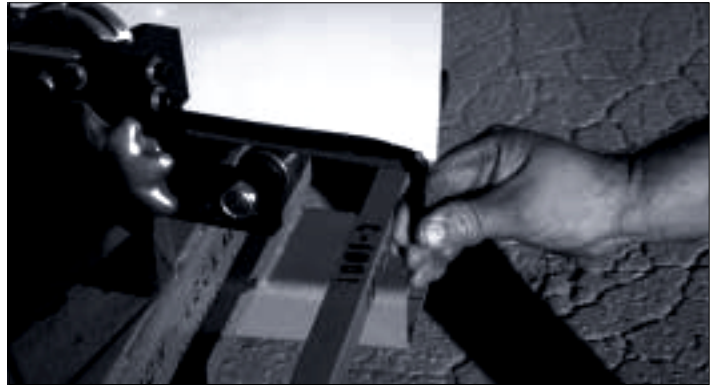
(Fig. 1) The vinyl must first be folded down over the panel to hold it in place so that it does not creep back as the panel is being formed.
