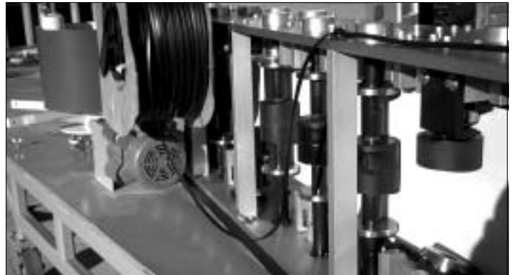
(Fig. 2) If the vinyl appears to be hanging up and is not being applied to the panel properly, it may be necessary to keep slack in the strip of vinyl as it comes off the vinyl coil on the side of the rollformer.
