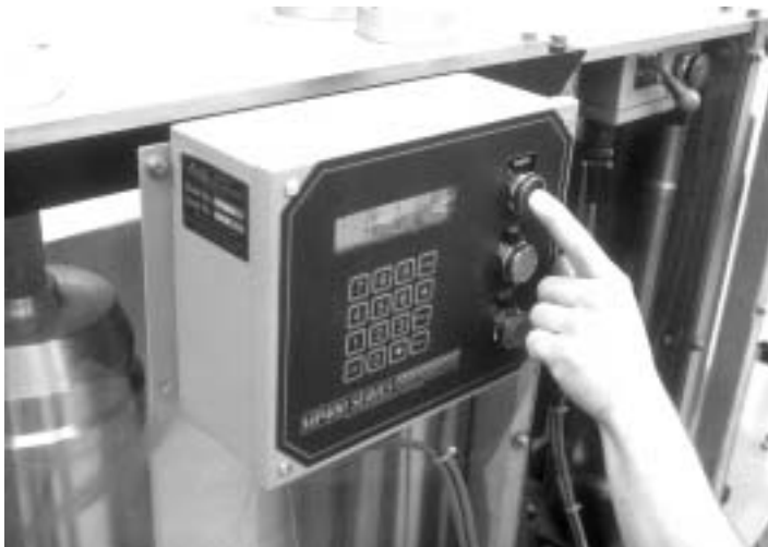
FIG. 4: PRESS THE "RUN" BUTTON TO VERIFY THE OPERATION OF THE COMPUTER AND TO BEGIN PRODUCING PANELS.
