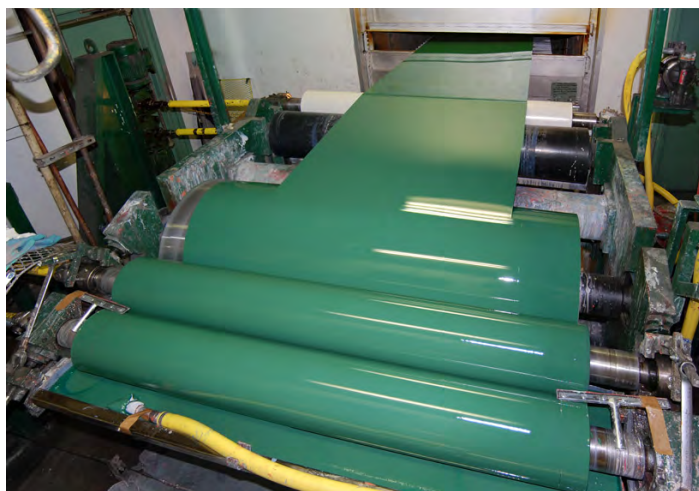
Berridge owns and operates its own modern continuous coil coating line in San Antonio, Texas, painting both 48" and 42" wide Galvalume® master coils.
