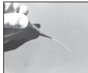
Fig. 4: Apply a fine line of paint to scratch area only - do not overpaint or blend.
