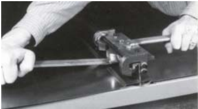
FIG. 1 - USE THE SINGLE-LOCK HAND CRIMPER FIRST...
