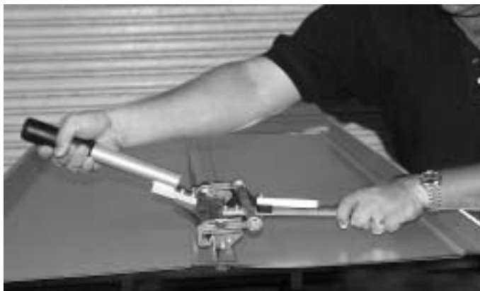
FIG. 2 - ...THEN COMPLETE HAND CRIMPING WITH THE DOUBLE-LOCK HAND CRIMPER
