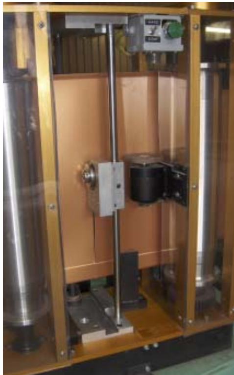
Clean vertical cut by rotary blade of Automated Shear
